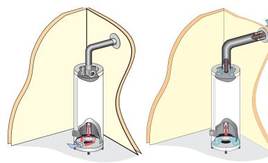
Fan-assisted water heater: The fan allows horizontal venting. The water heater may be open combustion or sealed combustion.
