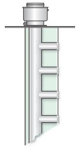
Multifamily exhaust ventilation system: Many multifamily buildings have vertically ducted exhaust ventilation systems with registers opening to kitchens and bathrooms on each floor.
