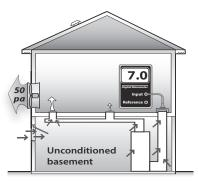
**Problem return register:** A pressure reading of 7 pascals indicates major air leakage near the tested register.
