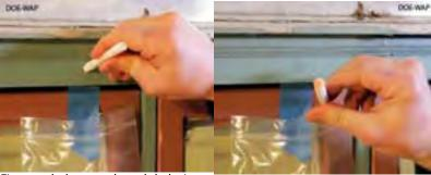
First, crush the capsule and shake it to mix ingredients. Then swab the sample for 30 seconds.
