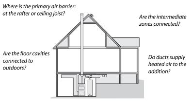
Is the half-basement inside or outside the air barrier? Is this space heated?
