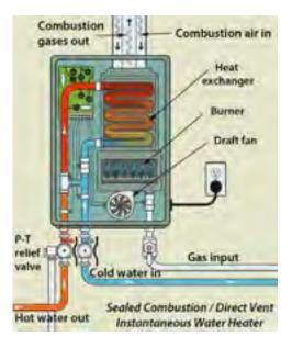
Heat pump water heater: This heat pump water heater has the heating coil (condenser) surrounded by the domestic water. Sealed-combustion on-demand water heater: These water heaters have a small market share and save around one-third of energy used by the best storage water heaters. Table 10-7: Comparison of Advanced Water Heaters
