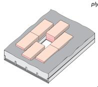
**Batts form attic-insulation dam:** Where head space is limited, fiberglass batts are a good choice for a low-profile insulation dam.
