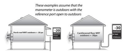
**Porch roof test:** If the porch roof were outdoors, the manometer would read near 0 pascals. We hope that the porch roof is outdoors because it is outside the insulation. We find, however, that it is partially indoors, indicating that it may harbor significant air leaks through the thermal boundary.
