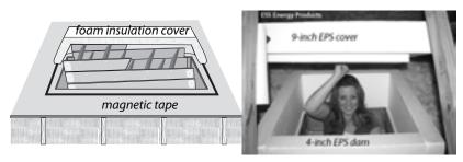
**Manufactured pull-down-stair covers:** Manufacturers provide insulated stair covers for use with walkable attic floors or with dams to be surrounded by fibrous insulation.
