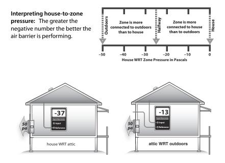
House-to-attic pressure: This commonly used measurement is convenient because it requires only one hose. Attic-to-outdoors pressure: This measurement confirms the first because the two add up to –50 pascals.
