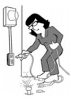
**Electrical safety:** Maintain cords in good condition. Use ground-fault-circuit interrupter (GFCI) cords for outlets in wet conditions.
