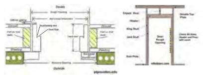
**Door anatomy:** The door and its frame fit into a rough opening. The door jamb matches the wall thickness and attaches to casing on the interior and exterior of the wall.
