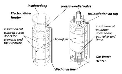
**Water heater insulation:** Insulation should be installed carefully so it doesn't interfere with the burner, elements, draft diverter, FVIR combustion intake, or pressure relief valve and discharge line.
