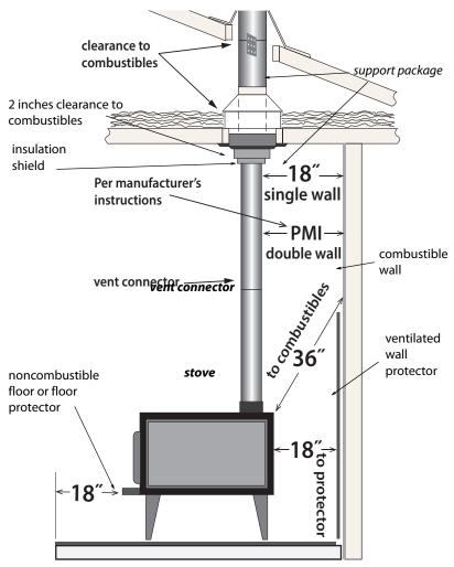
**Wood-stove installation:** Wood-stove venting and clearances are vitally important for wood-burning safety. Read manufacturer's instructions for the stove and its venting components.
