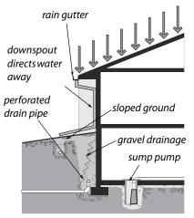
**Stopping water intrusion:** Take all necessary steps to protect homes from water intrusion.
