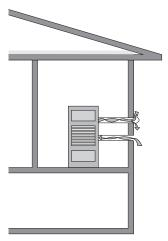
Sealed combustion heaters: Sealed-combustion furnaces prevent the air pollution and house depressurization caused by some open-combustion furnaces.
