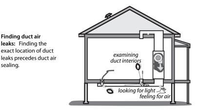
1. Use the air handler blower to pressurize supply ducts. Closing the dampers on supply registers temporarily or partially blocking the register with pieces of carpet, magazines, or any object that won't be blown off by the register's airflow increases the duct pressure and make duct leaks easier to find. Dampening your hand makes your hand more sensitive to airflow, helping you to find duct air leaks.
