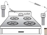
**CO from range and oven:** Measure CO at oven in undiluted flue gases. Measure ambient CO in the area of the range, but not directly above the burners or oven vent.
