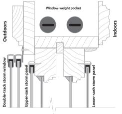
Optimized double-hung window: An exterior aluminum storm window plus storm window panels on the window sashes create triple glazing in this doublehung window.
