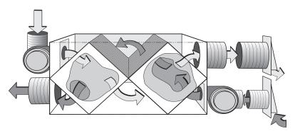
**Heat-recovery ventilator:** Heat from the exhaust air heats a plastic or aluminum heat exchanger, which in turn heats the fresh intake air. Two matched fans provide balanced ventilation.
