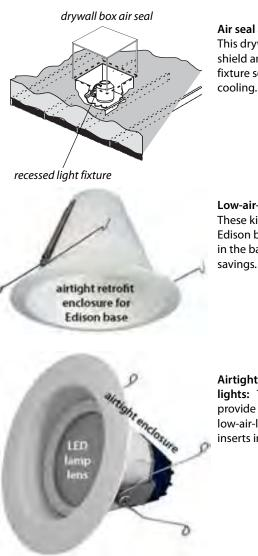
Air seal and shield for non-IC can: This drywall box is an insulation shield and air seal, but allows the fixture some air circulation for cooling.
