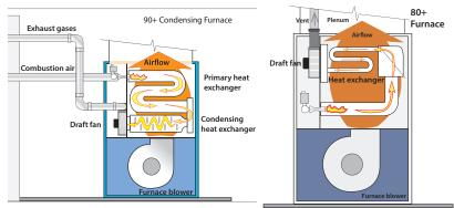
**90+ Gas furnace:** A 90+ furnace has a condensing heat exchanger and a stronger draft fan for pulling combustion gases through its more restrictive heat exchanger and establishing a strong positive draft. **80+ Gas furnace:** An 80+ furnace has a restrictive heat exchanger and draft fan, but has no draft diverter and no standing pilot light.
