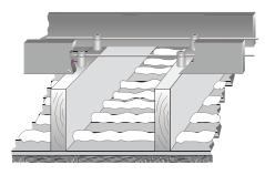
Shielding knob and tube: If you can't decommission knob-and-tube wiring, you may construct a dam to shield the wiring from insulation.
