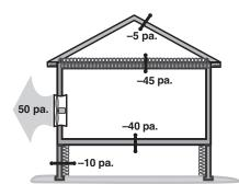
Pressure measurements and airbarrier location: The air barrier and insulation are aligned at the ceiling. The crawl-space pressure measurements show that the floor is the air barrier and the insulation is misaligned — installed at the foundation wall. We could decide to close the crawl space vents and air seal the crawl space. Then the insulation would be aligned with the air barrier.
