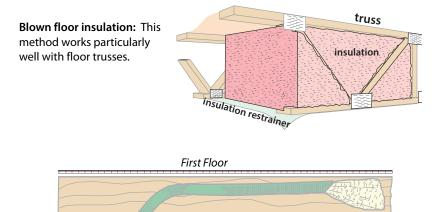
**Blowing floor cavity:** Uninsulated floor cavities can be blown with fiberglass or rock wool insulation, using a fill tube.
