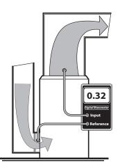
Static pressure and temperature rise: Measure static pressure and temperature rise across the new furnace to verify that the duct system isn't restricted. The correct airflow, specified by the manufacturer, is necessary for high efficiency.
