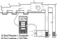
Total duct air leakage measured by the duct blower: All registers are sealed except the one connecting the duct blower to the system. Pressurize the ducts to 25 pascals and measure airflow.
