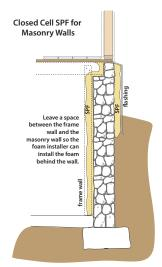
2-part foam sprayed on rubble masonry: Installers insulate rubble masonry walls on the interior or exterior with sprayed plastic foam. On the interior, they cover the foam with drywall.
