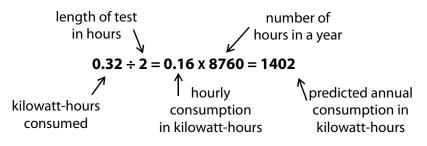
**Refrigerator consumption example:** In this example, a 2-hour measurement was performed. During this time, the appliance consumed 0.32 kilowatt-hours of electricity, or 0.16 kilowatt-hours per hour. The annual total of 1402 kilowatt-hours, calculated above, is well beyond the 450 kilowatt-hours per year consumed by today's most efficient refrigerators.
