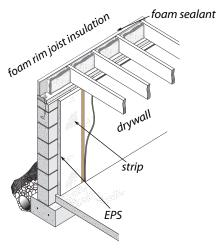
**2-inch foam board with plywood strips:** Installers fasten foam to the foundation wall using built-in strips. They then attach the drywall to the strips in the foam.
