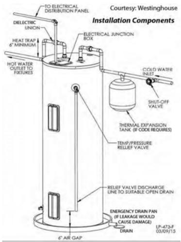
**Storage water heater installation:** The SWS requires these components on new-water-heater installations.
