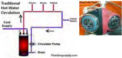
Hot-water re-circulation: Most multifamily hot-water circulation systems return cold water to the water heater and supply hot water to the distribution pipes.
