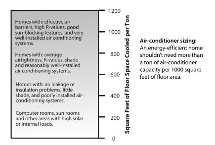
The cooling-cost reduction strategy should focus on making the home more energy efficient and making the air conditioner work more efficiently. Making the home more efficient involves shading, insulation, and air-leakage reduction. Making the air conditioner more efficient involves duct sealing, duct insulation, and a quality installation.
