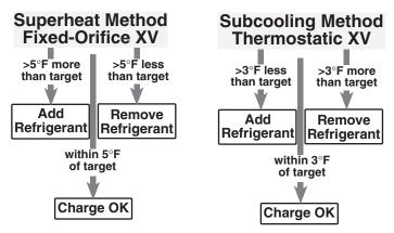
**Charge-checking:** Two methods help technicians judge whether the charge is correct. The remedy for incorrect charge is to either add or remove refrigerant.
