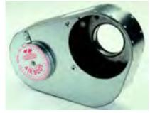
**Combustion air boot:** This metal boot attaches to the air intake of a power burner to provide combustion air from outdoors.
