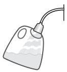
$60 \sec \div \frac{1 \text{ gal}}{15 \text{ sec}} = 4 \frac{\text{gal}}{\text{min}}$
