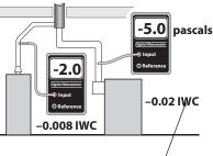
Measuring draft:Measurepascalschimney draft downstream of the<br/>draft diverter.
