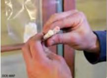
Red means lead-positive and white means lead-negative.
