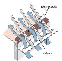
Ventilation pathways: Install baffles or chutes in every roof bay where soffit or eave venting exists.
