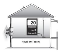
Bedroom test: This bedroom pressure difference may be caused by its leaky exterior walls or tight interior walls, separating it from the main body of the home. This test can determine whether or not a confined combustion zone is connected to other rooms.
