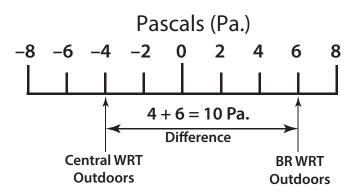
**Measuring unbalanced airflow:** The distance on a number line represents the difference in pressure between the central zone and the bedroom.
