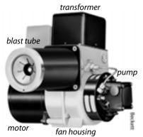
**Oil Burners:** Oil burners are power burners that atomize the oil by pumping it through a nozzle. A blower forces combustion air into the oil mist. Electrodes powered by a transformer light the mixture.
