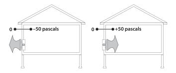
Conducting the Blower-Door Test
